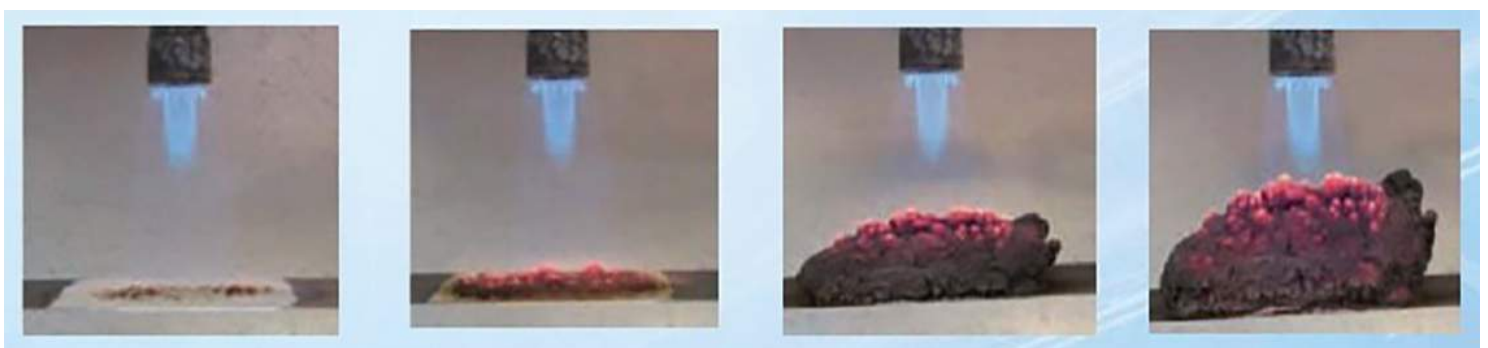
Coating just touched by flame
