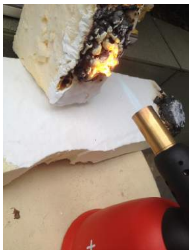
Polyurethane foam insulation protected with Top Firestop ® after 1 hour
